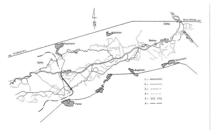
Fig. 1. Hydrographic network in the Narew Valley (Rzędziany-Żółtki section): 1 – The new channel of the Narew river, 2 – Old channels filled with water, 3 – Dry old river channels or filled with a small amount of stagnating water, 4 – Old river channels marked on the 1976 topographic map, 5 – Weirs and gates, 6 – Border of Narew National Park (NPN)
